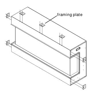
5. Make an opening for the fireplace according to requested measurement.
