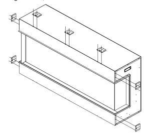
5. Make an opening for the fireplace according to requested measurement.
