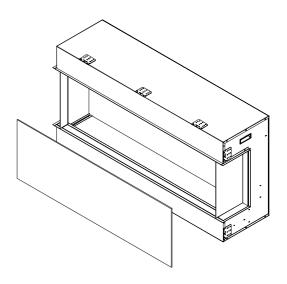
2. After the brackets are removed, the front glass panel will fall down automatically.
