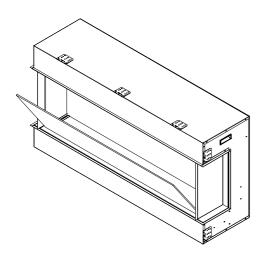
Installing the fire glass media. Pour the fire glass media into the tray as shown below.
